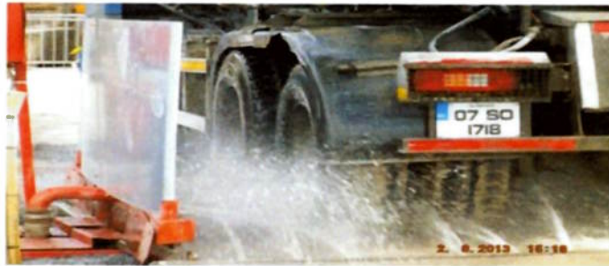
Figure 8 – Typical Wheel Washing Facility
